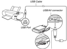
Making sure that the ▼ mark on the camera is aligned with the ▲ mark of the USB cable plug, connect the cable to the camera.
